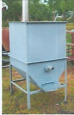
Figure 1. PhilRice continuous rice hull carbonizer.
