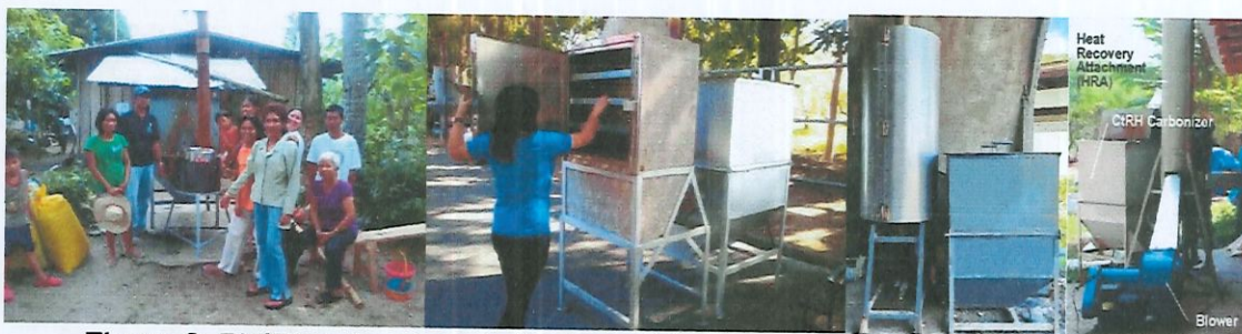
Figure 2. PhilRice developed attachment to recover heat from the carbonizer.
