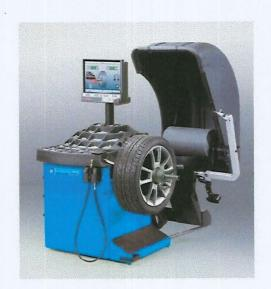
Wheel balancing alignment machine Rim Diameter, 10" - 24", 10" - 24" ; Rim Width, 1.5"  $\sim$  20", 1.5"  $\sim$  20" ; Balance Speed, 200 rpm, 200 rpm ; Max Wheel Weight, 65 kg, 65 kg ...
