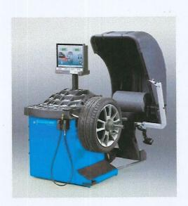
Wheel balancing alignment machine Rim Diameter, 10" - 24", 10" - 24"; Rim Width, 1.5"  $\sim$  20", 1.5"  $\sim$  20"; Balance Speed, 200 rpm, 200 rpm; Max Wheel Weight, 65 kg, 65 kg ...
